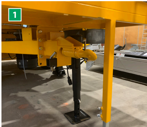
1 Bogie trailer The batching plants are installed on a joint twin-axle bogie in a welded steel frame. The draw hook is adjustable in height and can be dismantled, which helps to prevent theft.
