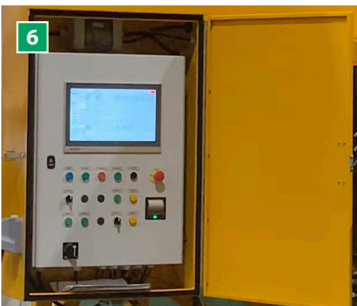
6 Control System Possibility of manual, semi-automatic and automatic operation and PC interface. No previous knowledge is required and can be delivered with the language version desired. Stores 50 recipes. Dosing accuracy: +/- 0,5 - 2%
