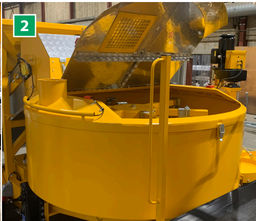
2 Pan mixer Pan mixer made in hard-wearing Hardox steel. B1800 and B2200 have an internal lining of replaceable, sectioned wearing plates. They are equipped with a gear motor for optimized effect, automatic radial opening, inlet for cement auger, and inspection hatches.
