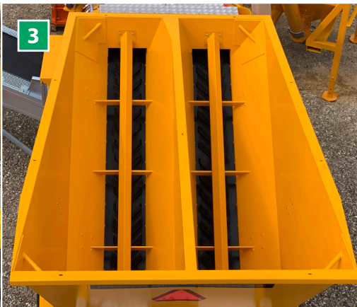
3 Hopper Integrated twin hopper for two types of aggregate. Each hopper holds 2 x 2.4 m 3 . It is made in an all-welded steel plate with reinforced corners and two separate feeding belts for the dosing of aggregates.
