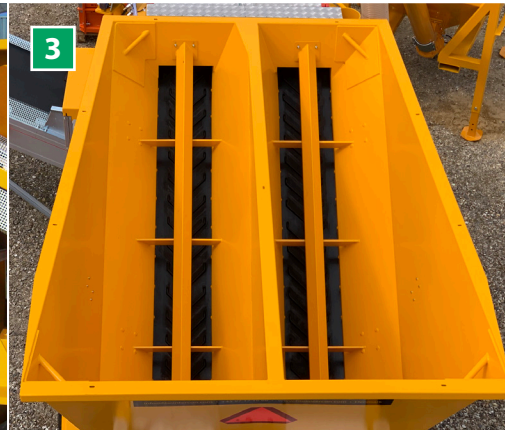
3 Hopper Integrated twin hopper for two types of aggregate. Each hopper holds 2 x 2.4 m 3 . It is made in an all-welded steel plate with reinforced corners and two separate feed belts for the dosing of aggregates.
