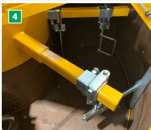
4 Mixing arms and side scrapers Adjustable mixing arms and side scrapers in steel and hard PVC. Equipped with safety bolts to prevent large stones from seriously damaging the mixing arms.
