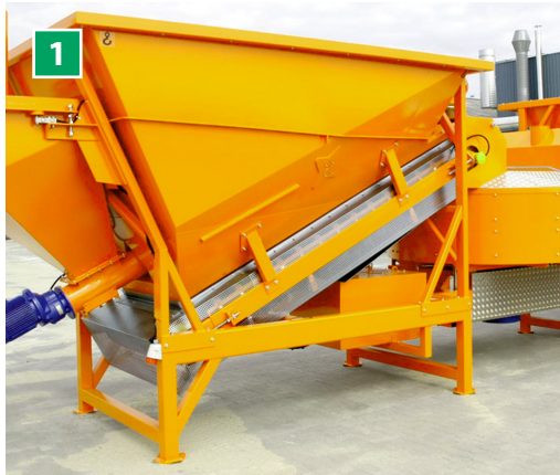
1 Steel frame The batching plant is mounted on a joint steel frame.
