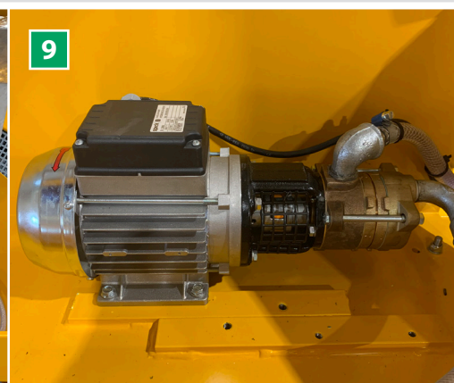
9 Additive pump (optional) High-quality dosing pump 0,25 kW for additive liquid, with 3/8" suction hose, check valve, and stainless steel strainer. Possibility for installation of 1 - 4 additive pumps.
