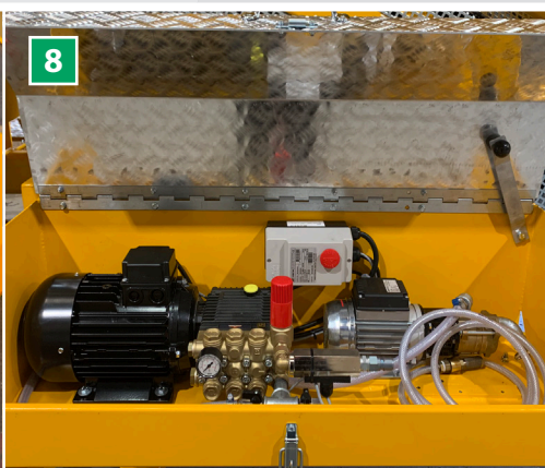
8 Equipment The standard FG-model is delivered with a high-pressure cleaner while the additive pumps are optional.
