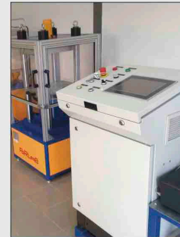
CONTROL EQUIPMENT FOR LAB Electric and hydraulic equipment for controlling each FORLAB test machine.
