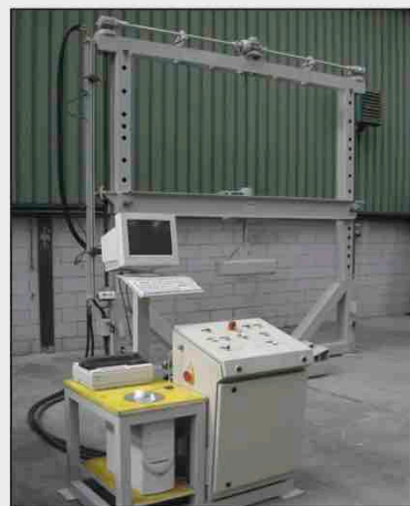
FLEXION TEST FOR CONCRETE PIPES
