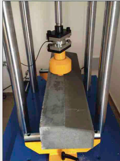
FORLAB F10T Press for flexion test Kerbstone 0 to 100 KN
