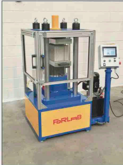
FORLAB C150T Press for compression test 0 to 1500 KN concrete test blocks, pavers, ....
