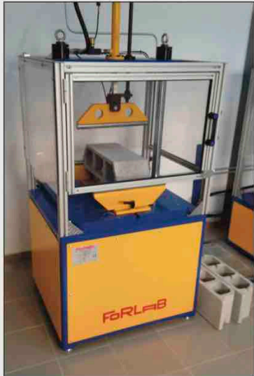
FORLAB F250K Press for flexion test Ceilings 0 to 2500 N
